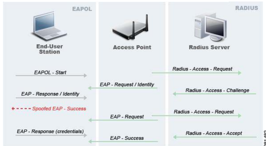
Figure 19-17 EAP-Success Protocol and EAP-Success Attack
