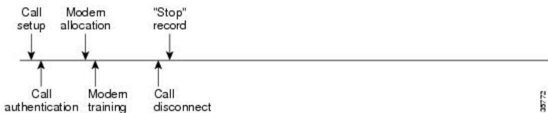
Figure 83: Modem Dial-In Call Setup Sequence With Call Disconnect Occurring Before User Authentication and With Resource Failure Stop Accounting Enabled
