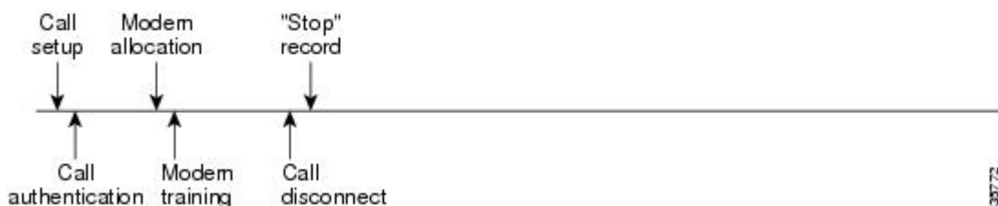
Figure 71: Modem Dial-In Call Setup Sequence With Call Disconnect Occurring Before User Authentication and With Resource Failure Stop Accounting Enabled
