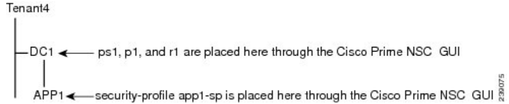
Figure 9: Cisco Prime NSC Organizational Hierarchy for a Tenant, Data Center, and Application
