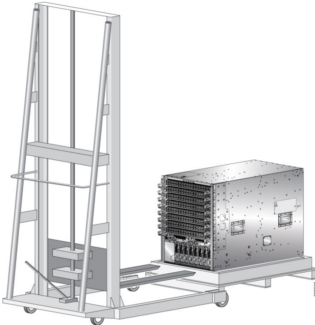
Figure 7: Align the Lifting Device in Front of the Chassis on the Pallet
