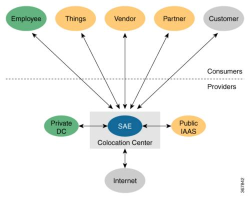
This is where SAE comes in. SAE offers the capability of virtualizing your network edge and extending it to colocation centers. SAE provides segmentation, virtualization, automation, and orchestration for your enterprise within a carrier-neutral facility.
