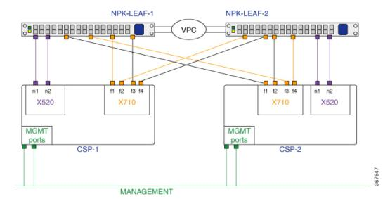
• Connect each CSP device to both the Nexus 9000 switches using two 10G ports in port-channel configuration. Each CSP device has four XL710 interfaces, which enable port channeling. Two of these ports must be connected to leaf 1 and two to leaf 2.
