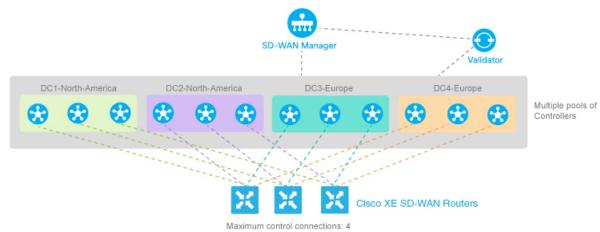
As is the case with any overlay network that has multiple Cisco SD-WAN Controllers, all policy configurations on all the Cisco SD-WAN Controllers must be the same.
