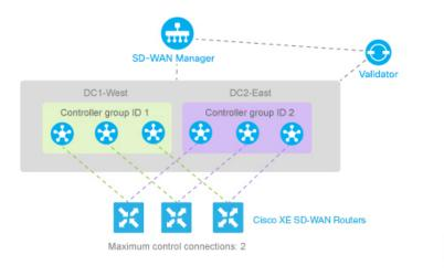
You configure the three Cisco SD-WAN Controllers in DC1-West with controller group identifier 1:
