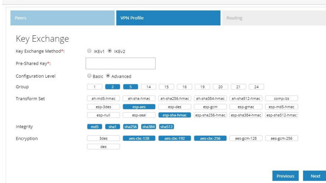
Figure 95 DMVPN Spoke Configuration (VPN Profile Advanced Options)
