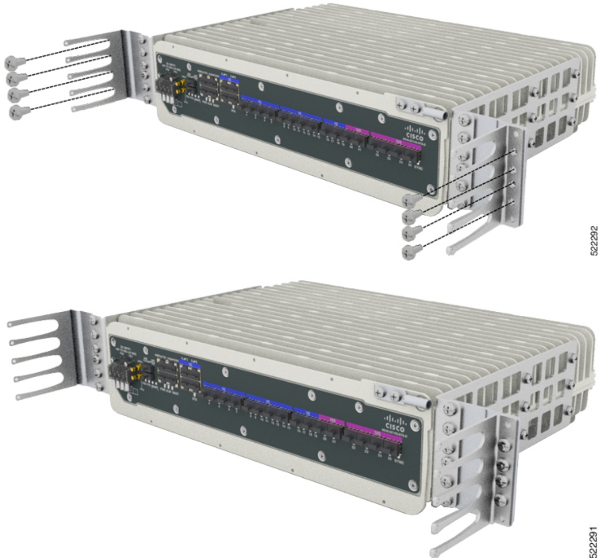
Figure 10: Cable Guide Installation For 23-inch Rack Brackets
