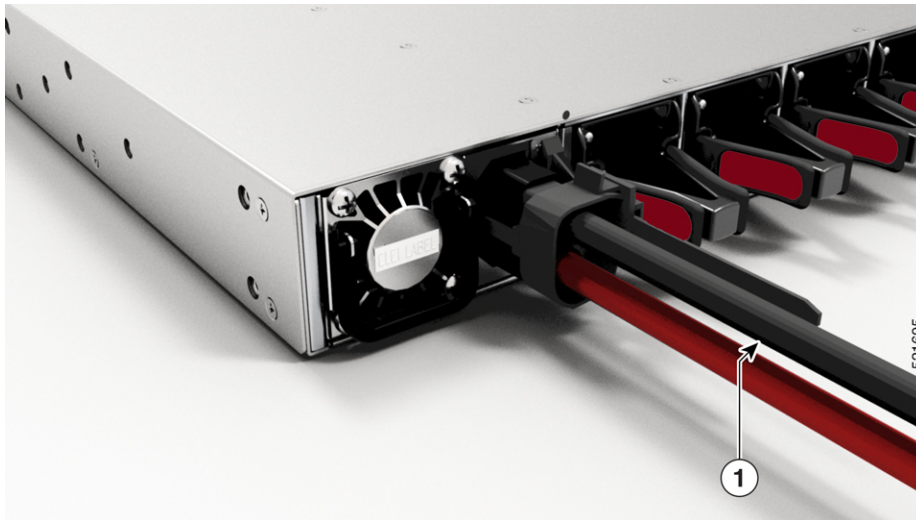
Figure 32: Connecting DC Power - Cisco 8111-32EH-0
