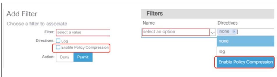
Figure 51 Enabling compression on filters
