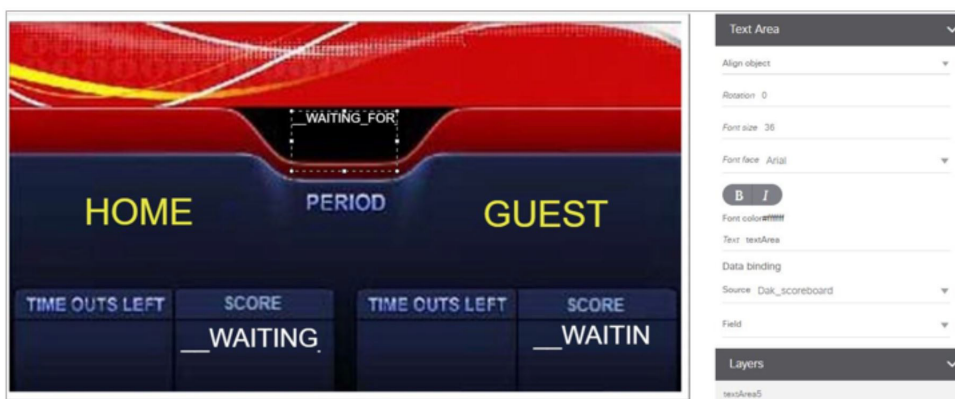
Figure 25 Period Data Field Binding for OES Ice Hockey Scoreboard Source
