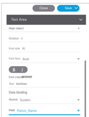
Figure 65 Binding the System Data Source and PatronName Data Field
