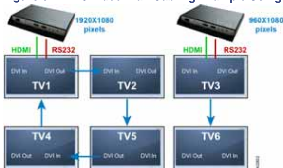
Figure 5 2x3 Video Wall Cabling Example Using TV Tile Matrix Functionality
