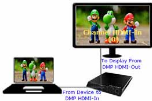
Figure 6 Local HDMI-In Pass-Through to Single TV Display
