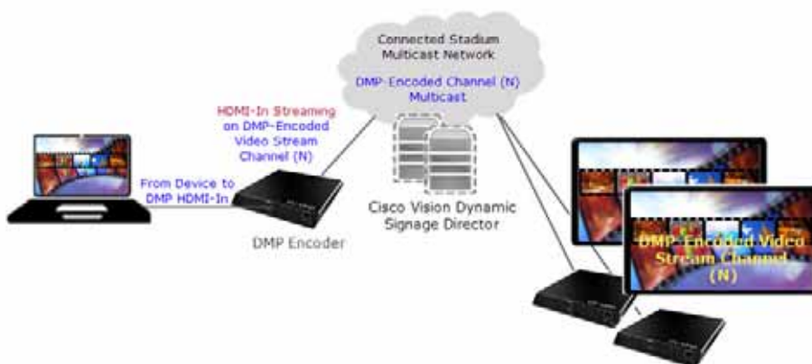
Figure 7 HDMI-In Streaming Example from Single DMP to Multiple DMPs
