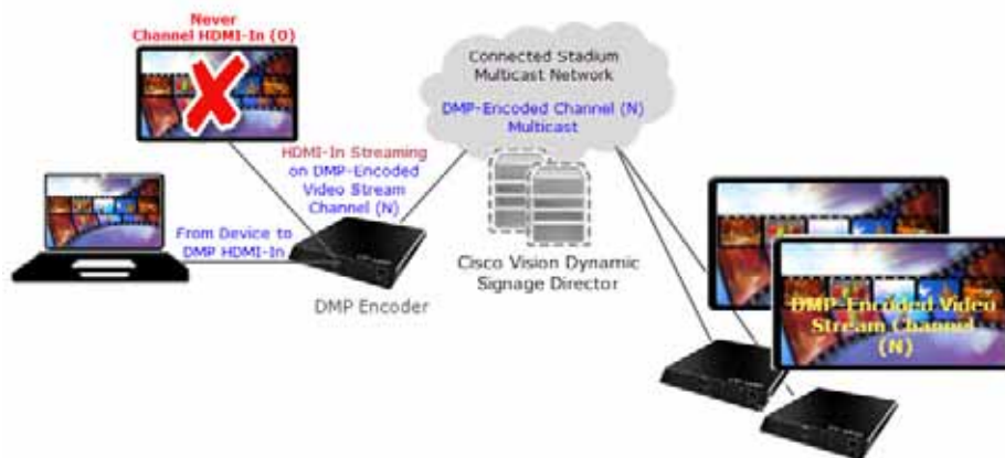
Figure 8 Unsupported DMP Encoder Configuration for HDMI-In Streaming
