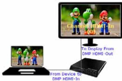
Figure 5 Local HDMI-In Pass-Through to Single TV Display
