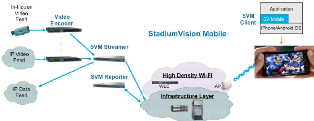
Figure 1 Cisco StadiumVision Mobile Architecture
