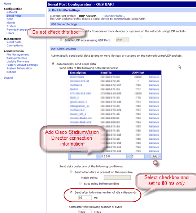
Figure 1 OES ISC9000 Configuration
