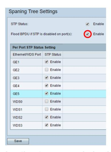
Step 4. (Optional) Under the Per Port STP Status Setting area, check the check boxes to enable STP on your preferred Ethernet/WDS port.
