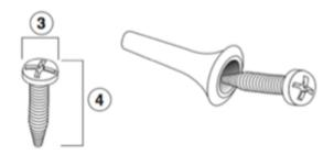
Step 5. Tighten each screw and leave a gap between the surface of the wall and the head of the screw.
