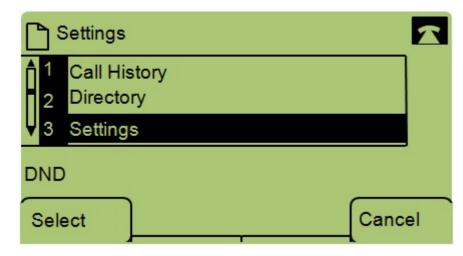
Step 2. Navigate to Settings and press Select using the soft-key.
