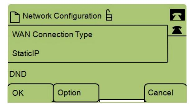
Step 6. Press Option to toggle between DHCP and Static IP.
