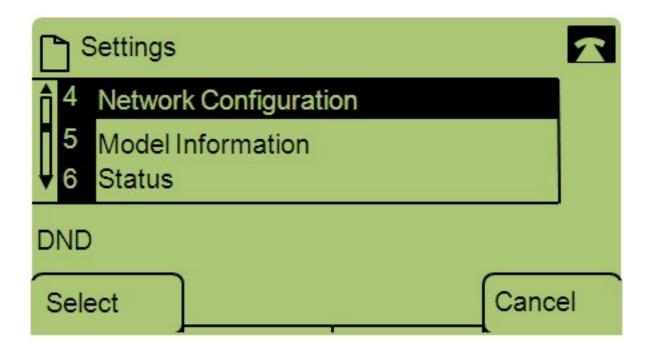
Step 3. Navigate to Network Configuration and press Select using the soft-key.
