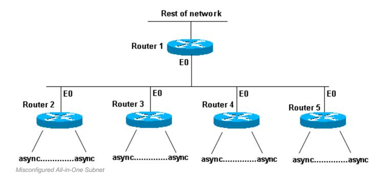
Routers 2 through 5 are access routers that each have several incoming asynchronous (or ISDN) connections. The network (192.168.1.0/24) is broken up into four pieces for these incoming users. Each piece is given to one of the access routers. Also, the asynchronous lines are configured **ip unnum e0**. Router 1 has static routes that point at the correct access router, and each access router has a default route points at Router 1.
