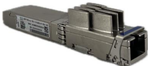
Figure 1. Cisco XGS-PON OLT SFP+ module
