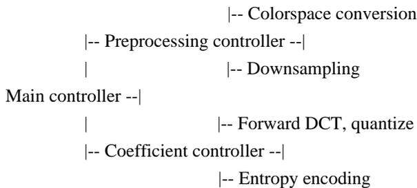
This sketch also describes the flow of control (subroutine calls) during typical image data processing. Each of the components shown in the diagram is an "object" which may have several different implementations available. One or more source code files contain the actual implementation(s) of each object.
