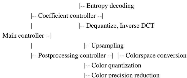
As before, this diagram also represents typical control flow. The objects shown are:
