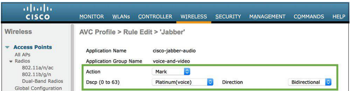
Figure 16. Adding rules to mark the application traffic types to the AVC Profile
