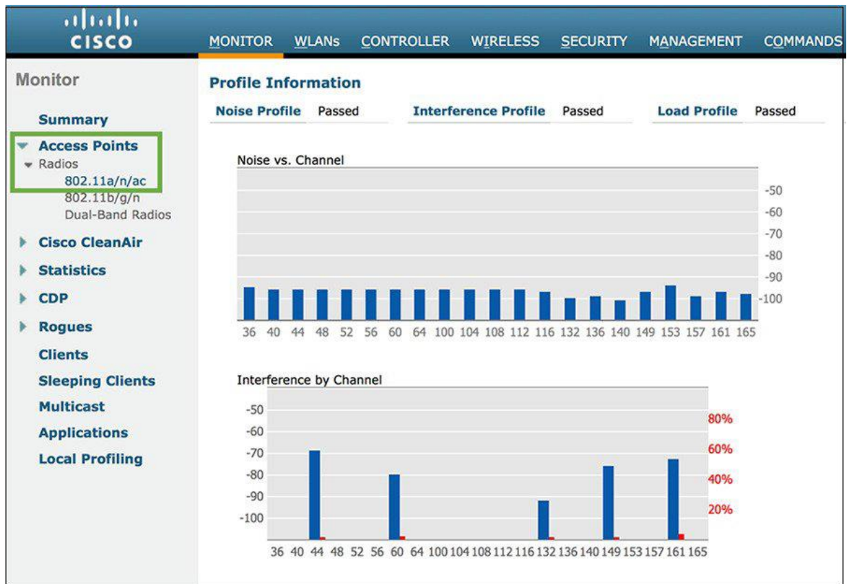
Figure 29. Checking AP Statistics to monitor the RF environment
