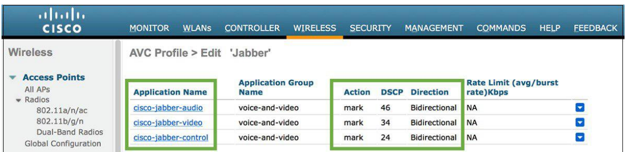
Figure 17. Verifying all the rules for the application traffic type associated to the AVC Profile
