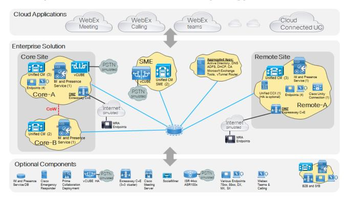
This test bed is designed to be very flexible and is built to meet specific test requirements. It provides a basic enterprise solution with a number of optional components, such as server applications, high availability, gateways, and UCS hardware. You can add or subtract these optional components wherever required.
