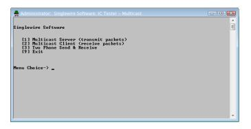
**Step 4** Enter **2** at the **Menu Choice** prompt and press the **Enter** key. The IC Tester - Multicast window refreshes, showing it initially failed to find multicast, but then detects it.
