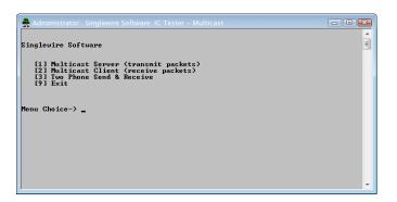
**Step 2** Enter **1** at the **Menu Choice** prompt and press the **Enter** key. The IC Tester - Multicast window refreshes, showing multicast packets being sent across your network.
