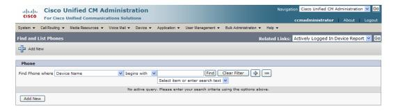
**Step 4** Use the dropdown menus and fields to locate the phone attached to the PC on which you downloaded Wireshark. Your results will appear below the fields.
