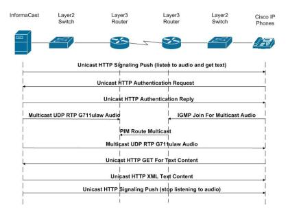
Now that you are familiar with the traffic flow created by InformaCast, you can use a protocol analyzer, such as Wireshark, to sniff the traffic on the network to see that multicast is enabled.
