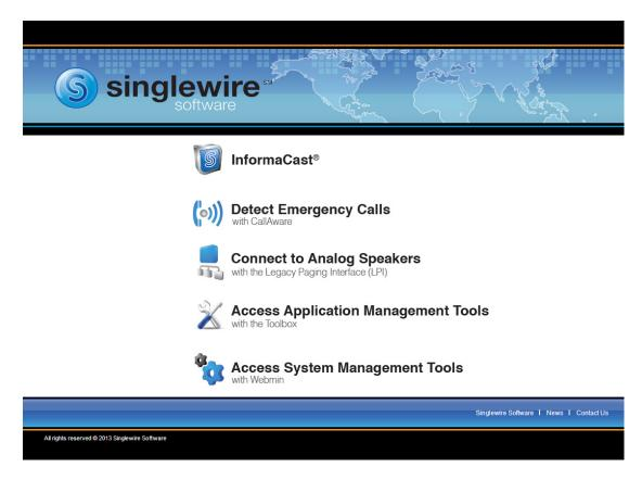
Step 2 Click the Access Application Management Tools with the Toolbox link. A separate tab/window opens to the Toolbox page.
