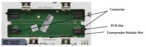
Important Note: Make sure that the transponder is inserted in the correct slot.
