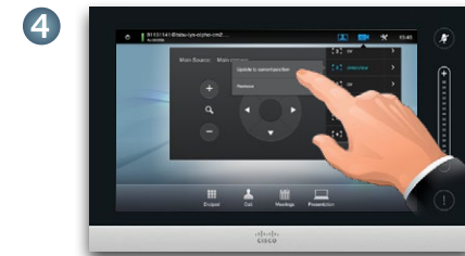
In the submenu tap Update to new position to put your changes into effect, or tap Remove to delete the selected preset.
