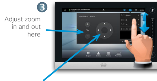
Adjust zoom in and out here Use these controls to define the direction in which the camera shall point (also known as Pan control).
