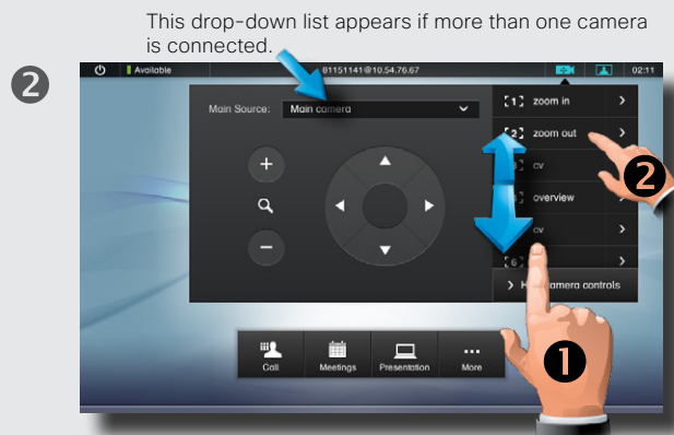
If needed, scroll to show the camera preset to be removed (1) and then tap > of that preset to expand the menu (2). If you have more than one camera connected to your system, you may choose camera.
