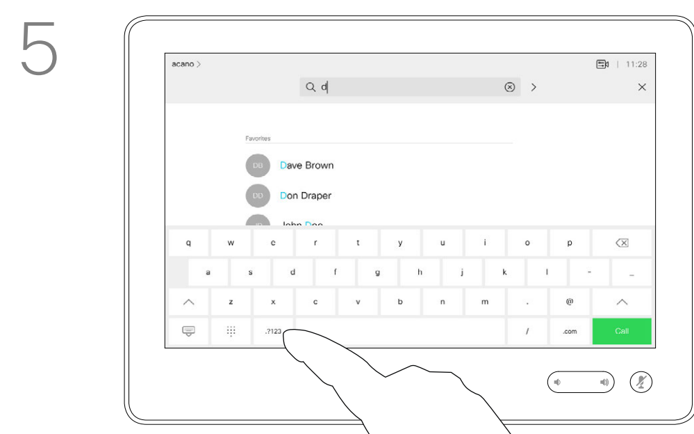
5 There is an extended numerical mode available, which also contains special characters. To toggle between the alphanumeric mode and the extended numerical mode tap the key in the lower left corner of the keyboard.
