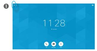
Starting from *Home* screen, use the **Cursor** keys on the remote control to select the Settings field in the upper left corner of the screen.
