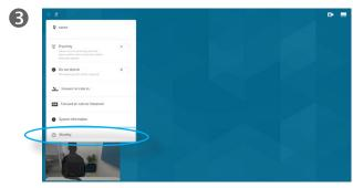
Use the **Down Cursor** button five times on the remote control to select *Standby*. If your system has Intelligent Proximity enabled you will need to press the **Down Cursor** button six times.
