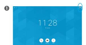
In a call or outside a call (as shown here), move cursor up to the upper right corner to the **Camera** icon. Press **OK** on the remote control.
