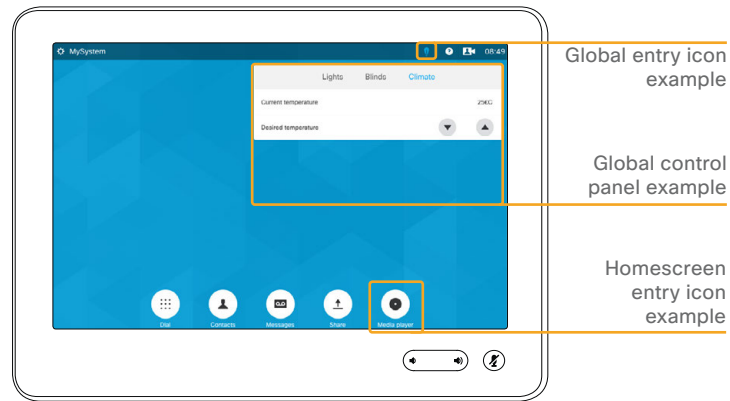
Example of Global and Homescreen in-room control panels on Touch 10. Any In-Call panel icons existing will be visible during calls only.
