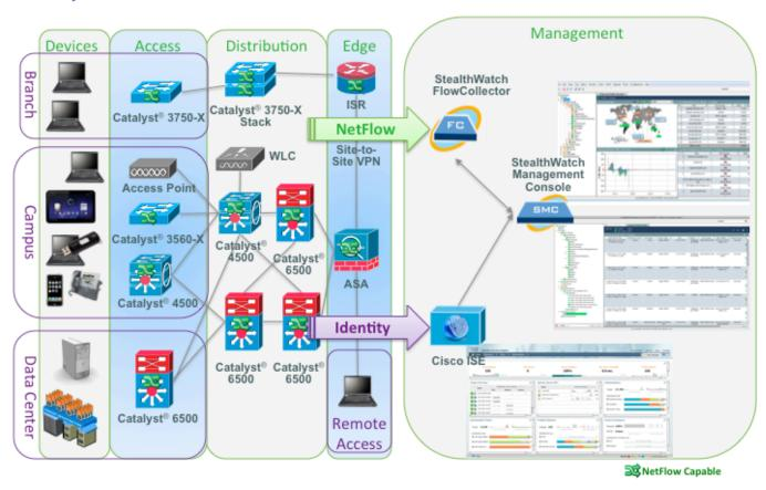
Visibility into network traffic is provided through NetFlow export from Cisco routers and switches while identity services, including the user name and profile information is provided through the
