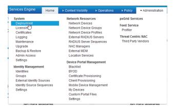
Click Edit under Deployment Nodes to set the properties of the ISE node where you want to activate pxGrid.
