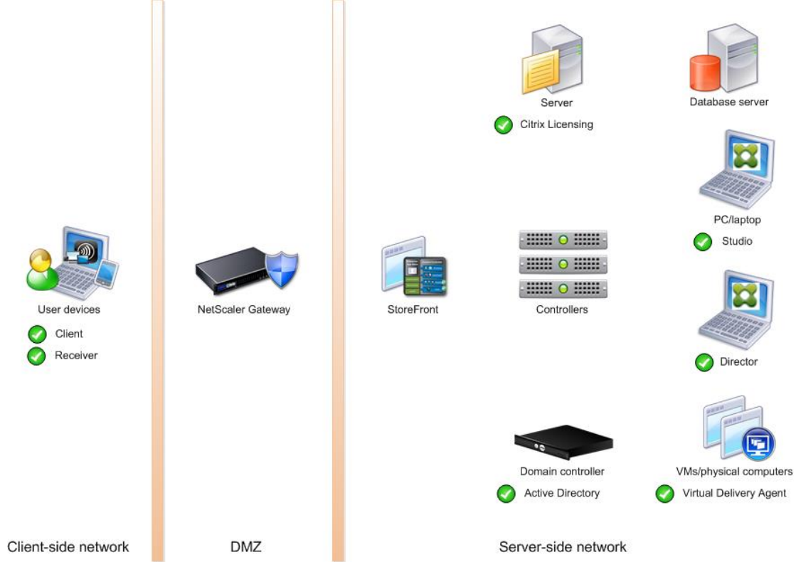
Figure 21 Example of a Distributed Components Configuration
