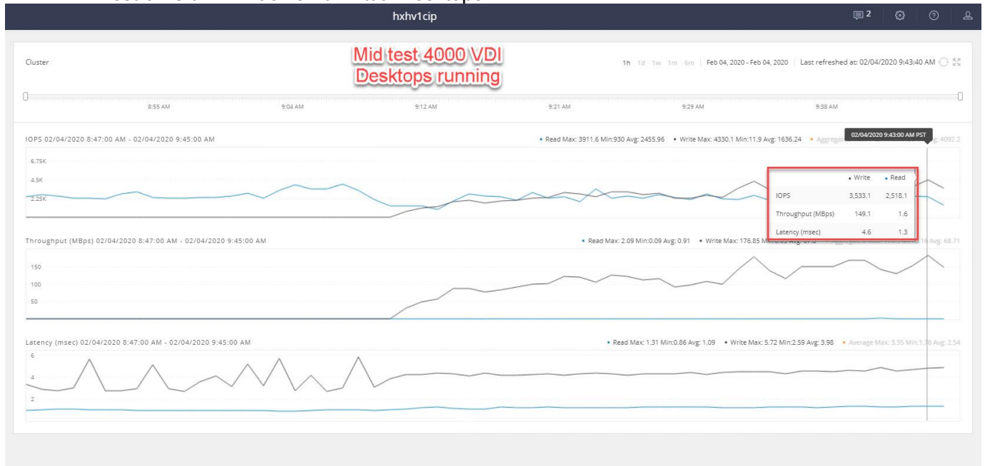
Figure 133 HyperFlex Cluster UI Performance Chart for Knowledge Worker Workload Running 4000 User Test on Citrix Windows 10 Virtual Desktops
