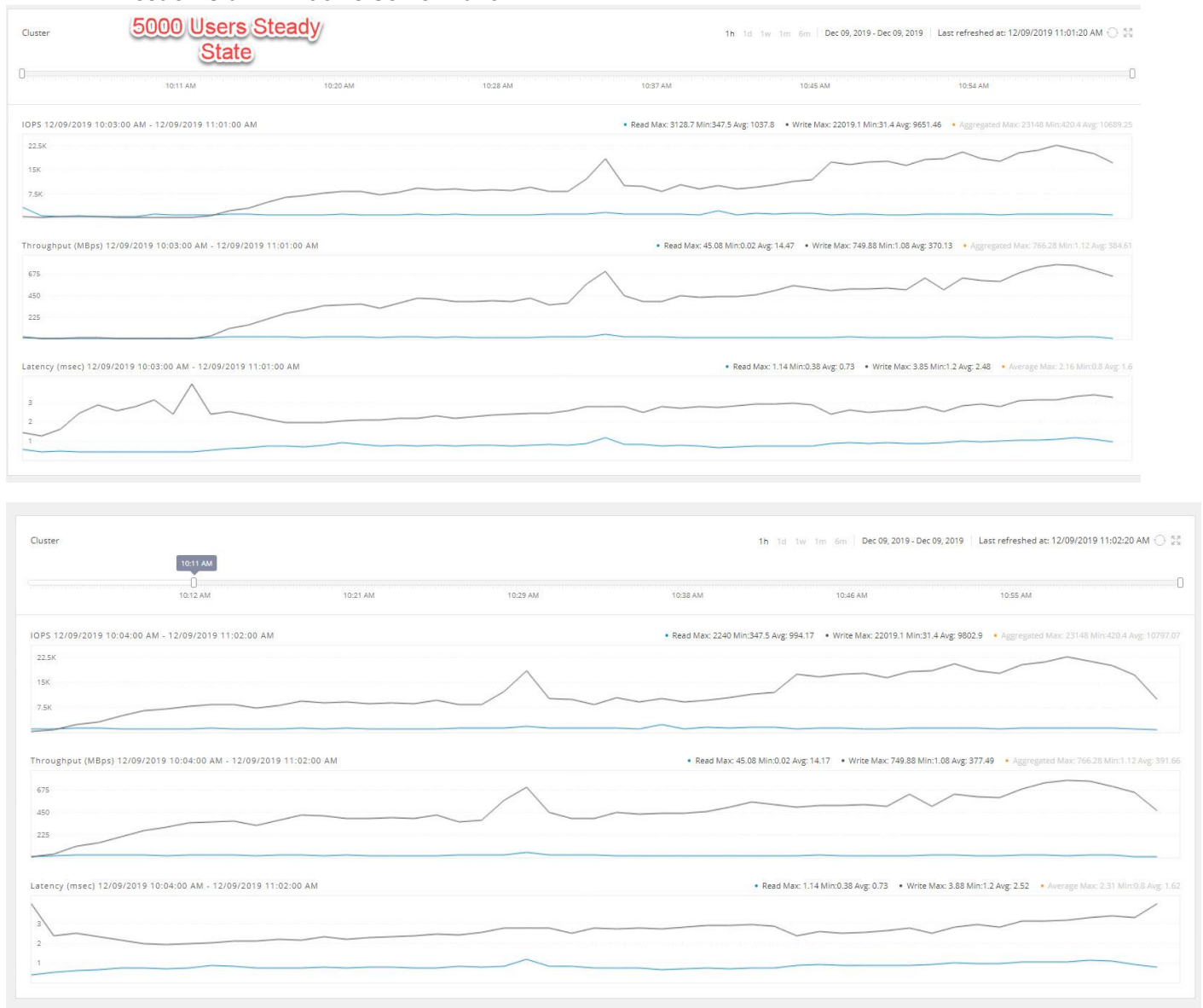
Figure 129 HyperFlex Cluster UI Performance Chart for Knowledge Worker Workload Running 5000 User Test on Citrix Windows Server 2019
