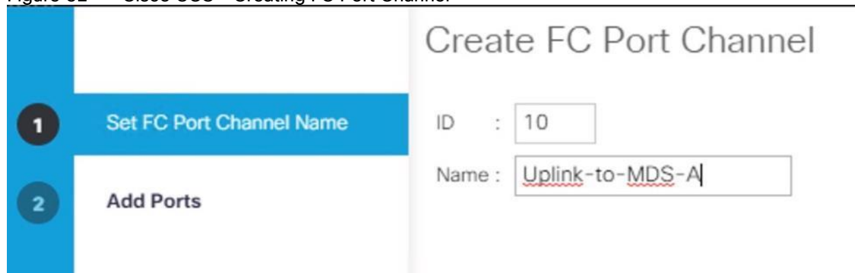
Figure 52 Cisco UCS - Creating FC Port Channel
