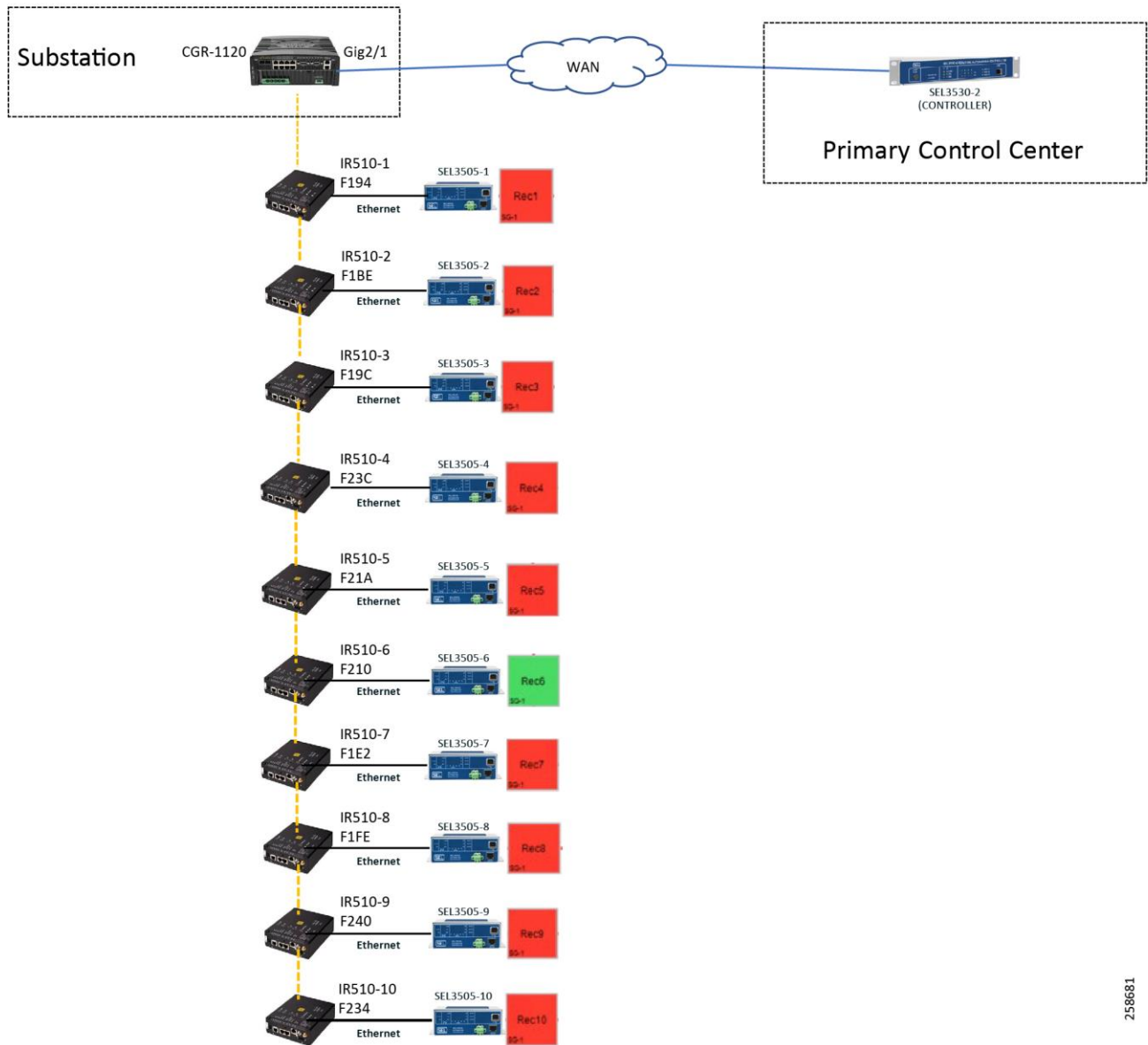
Figure 12. Rural SEL reclosers to Cisco RM device mapping diagram
