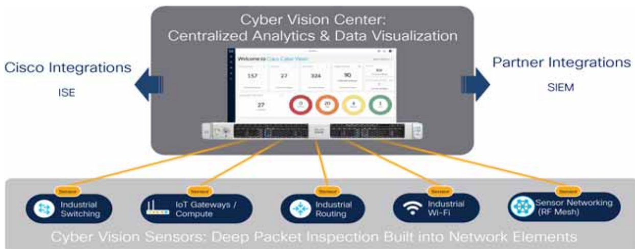
Figure 65 Cisco Cyber Vision Two Tier Architecture
