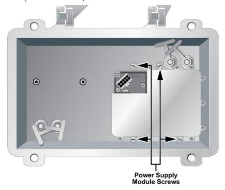
**4** Attach the 10-pin keyed connector of the power cable and harness to the power supply module.
