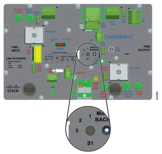
5 Adjust the AGC gain control potentiometer to match the level you measured in step 3.
