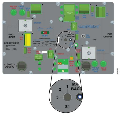
Adjust the AGC gain control potentiometer to match the level you measured in step 3.
