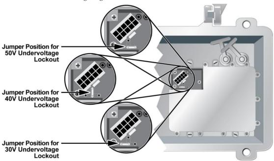
**Note:** The AC undervoltage lockout selector positions are also noted on the power supply.
