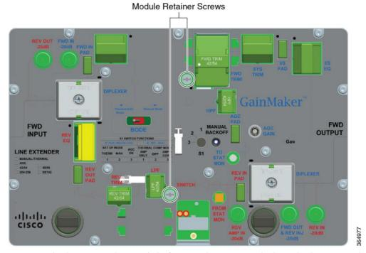
7 Remove the line extender module from its housing and place the line extender module on a secure surface.
