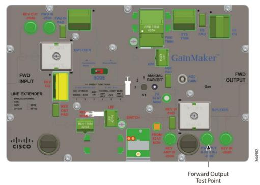
Measure and note the RF output level at the AGC pilot frequency.
