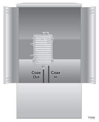
**Note:** The housing mounts to the bracket provided by the pedestal manufacturer.
