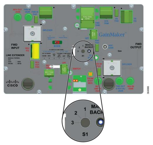
2 Insert the test probe into the -20 dB forward main output test point on the line extender.
