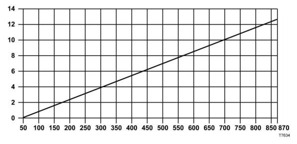
**Example:** If the line extender's 870 MHz output level is 47.5 dBmV with a linear operating tilt of 12.5 dB (from 50 to 870 MHz), the corresponding output level at 650
