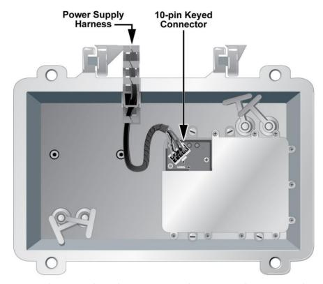
**Note:** The 10-pin keyed connector can be connected one way only. Be sure that the connector is installed securely to the power supply board.
