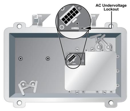
**2** Set the AC undervoltage lockout selector for your powering application as illustrated in the following diagram.
