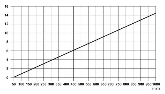
**Example:** If the line extender's 1 GHz output level is 49.0 dBmV with a linear operating tilt of 14.5 dB (from 50 to 1 GHz), the corresponding output level at 750 MHz would be 45.1 dBmV. This was found by taking the difference in tilt between 1 GHz and 750 MHz (14.5 – 10.6 = 3.9 dB). Then subtract the difference in tilt from the operating level (49.0 - 3.9 = 45.1 dBmV).
