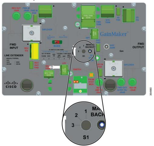
Turn the MANUAL BACKOFF potentiometer fully counterclockwise for maximum gain.
