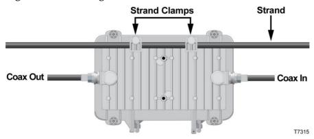
**Note:** Coax In may be switched with the Coax Out if you reverse the line extender module and feed the signal from right to left.
