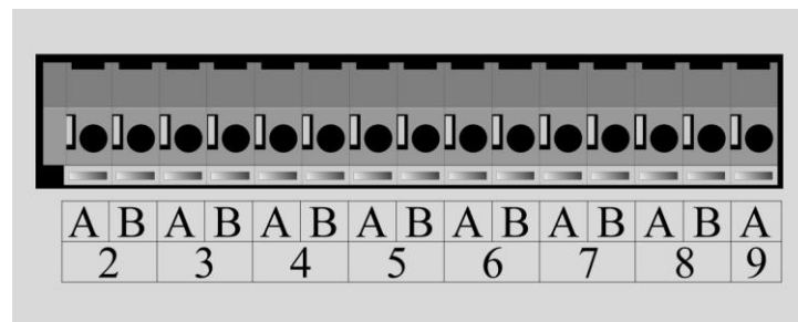
Close-up of Front Panel Terminal Strips
