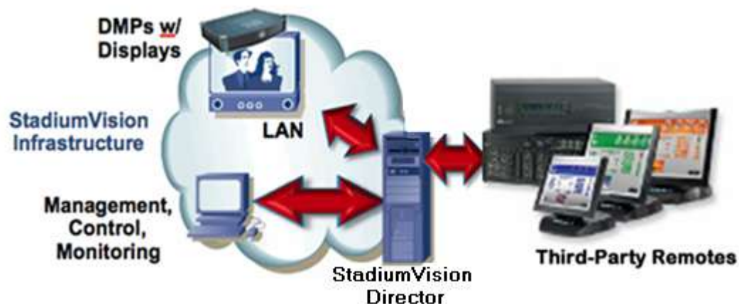
Figure 9. Local TV Control via a Third-Party Touch Panel
