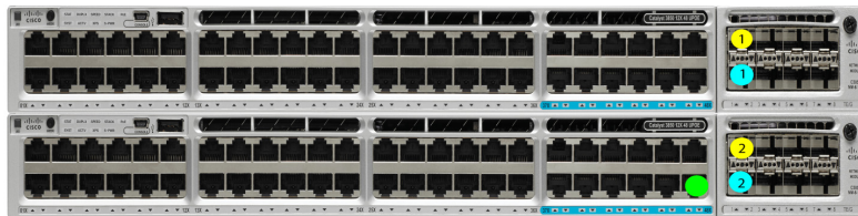
Dual 10/25GE ToR Switches (standalone or stacked)
